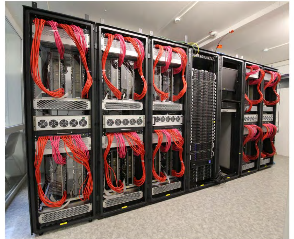
Brainscales 20 wafer machine. 4M neurons, 1B synapses
